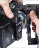
Make sure that the quick release on the V-Grip is open. The latch should point 90 degrees out from the grip. Place the V-Grip on the bracket on the XF camera body so it aligns with the XF hand grip and the contact pins integrates well into the connector recession.
