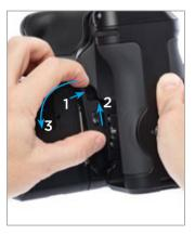
To remove the V-Grip, first press the top of the quick release hatch towards the front (1) Then push the quick release safety switch towards the top of the grip with your thumb. (2) Then use your index finger to flip the quick release latch 90 degrees out from the V-Grip. Remove the V-Grip.
